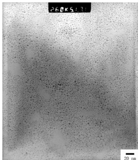
Figure 1. TEM image of gold nanoparticles at 260,000X.
