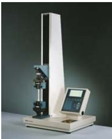
Figure 1 – Instron Tester: Tinius Olsen H5KS
