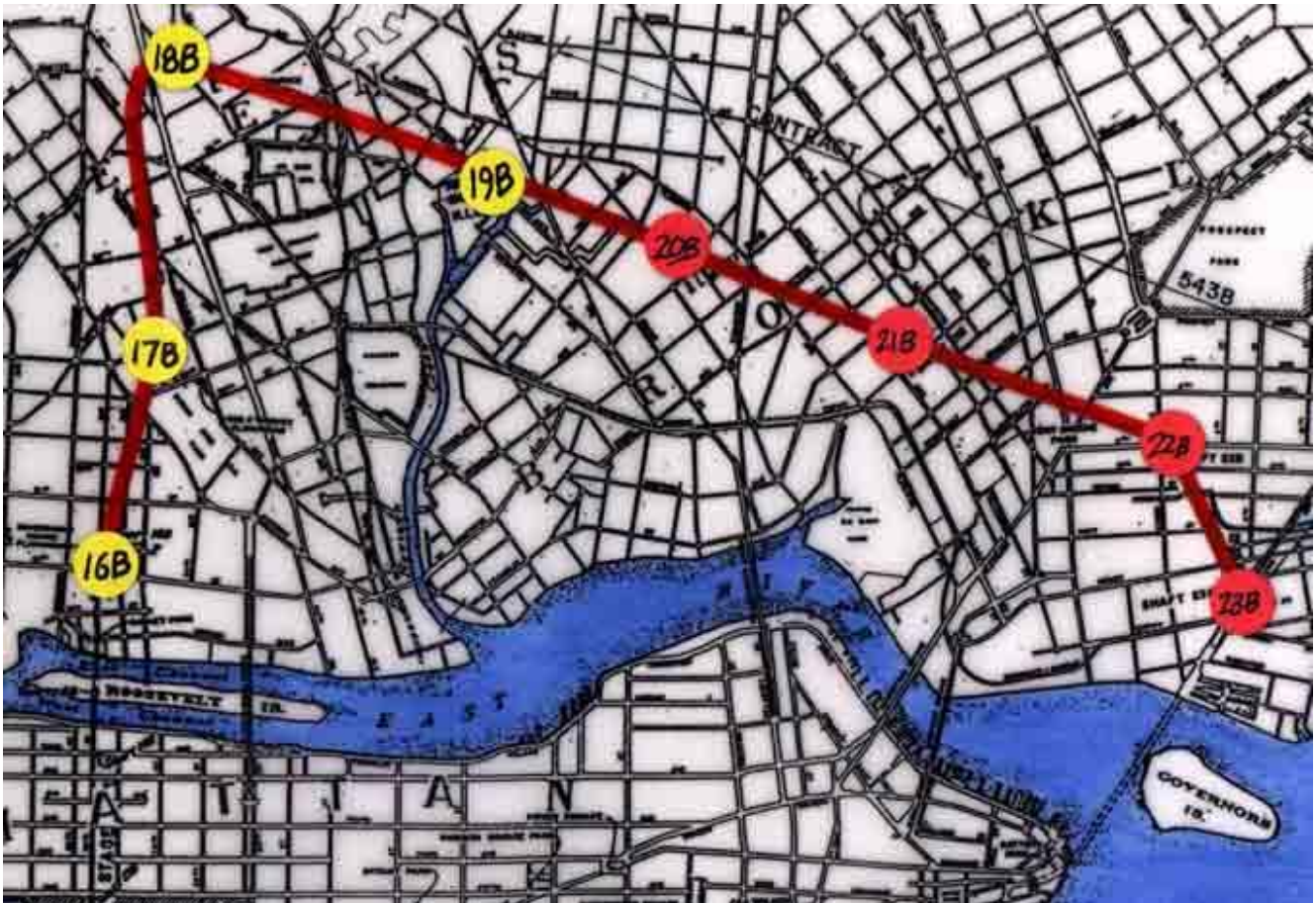
Figure 1 – Index map showing the plan view of City Water Tunnel #3, Stage 2. The positions of Brooklyn Tunnel (Shafts 23B to 19B) and the Queens Tunnel (Shafts 19B through 16B) are shown. North is toward the lower left.
