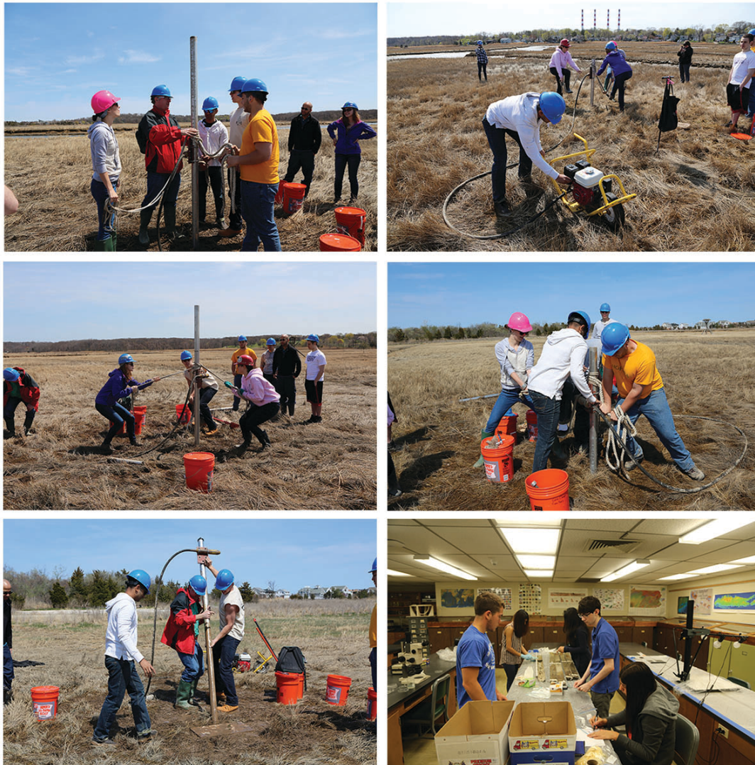
Figure 2. Photomontage illustrating the vibracoring process. From top left: positioning the hollow core tube, starting the motor to vibrate the core tube, driving the vibrating core tube into the marsh subsurface (middle row images), extracting the core, and splitting, photographing, and sampling the core.
