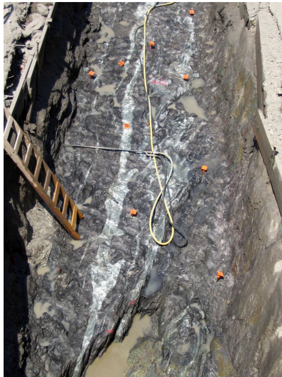
Figure 9 – Asymmetric F_3 z-fold in Walloomsac schist and calc-silicate unit showing NE-trend, steep axial plane foliation and transposition foliation with subvertical plunge. (CJM Digital image, 2008; near WTC Stop 13.)
