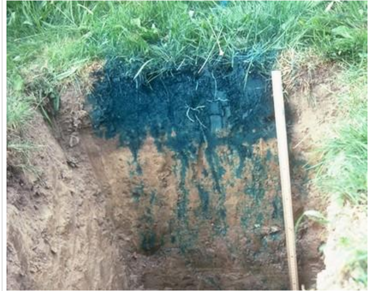
Figure 4: Notice how the nontoxic blue dye begins to trickle in less amounts when reaching the lighter soil.
