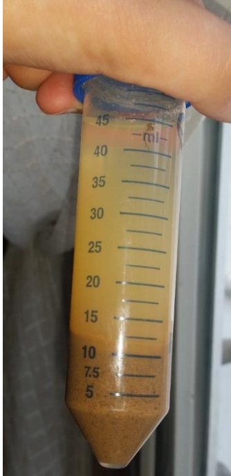
Figure 2: An example of how measurements were taken during grain size analysis using the centrifuge tubes.
