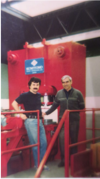
Yuriy Litvin with Tibor Gasparik and the USSA-2000 multi-anvil apparatus in the Stony Brook High-Pressure Laboratory.
